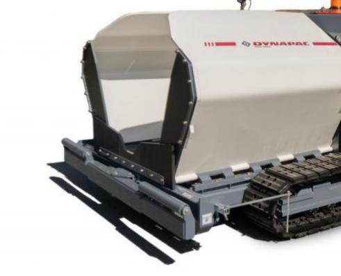
WEAR RESISTANCE, BOLT ON REPLACEABLE CONVEYOR FLOOR PLATE
