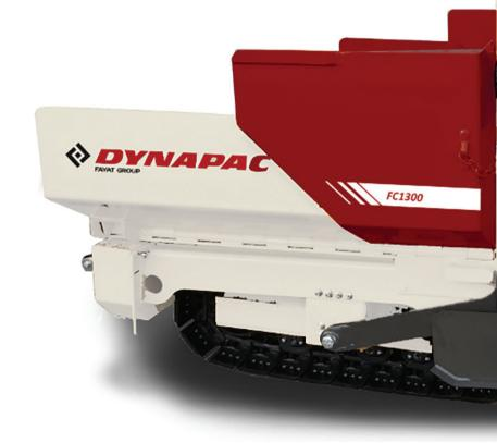
Dynapac FC1300C is designed to pave patch works, driveways and small lots. With tilt hopper and gravity feed design customers can easily unload the asphalt in to the auger chamber. The heavy duty VF0813C screed weighs 2000 lbs (900 kg) for best pre-compaction and heated with propane gas. Simple operator controls with cable drive and gauges makes it very easy to learn and operate the paver.
