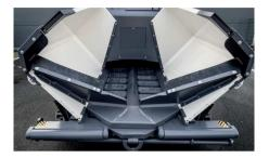
CHOOSE YOUR HOPPER MODEL A specially shaped hopper allows you to receive and store material more efficiently, thus avoiding physical and thermal segregation. Chamfers in the hopper's corners prevent the material from sticking and guide it directly to the feeding conveyor in the middle of the machine.
